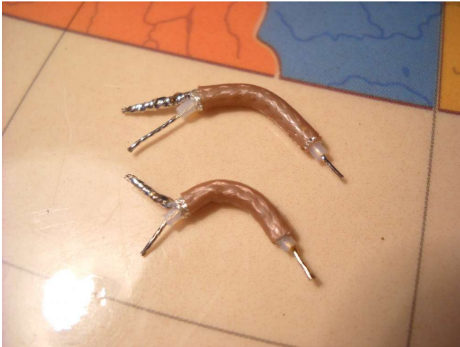
Preparation of the two small pieces of coaxial cable for the Faraday-shielded "primary" windings.
